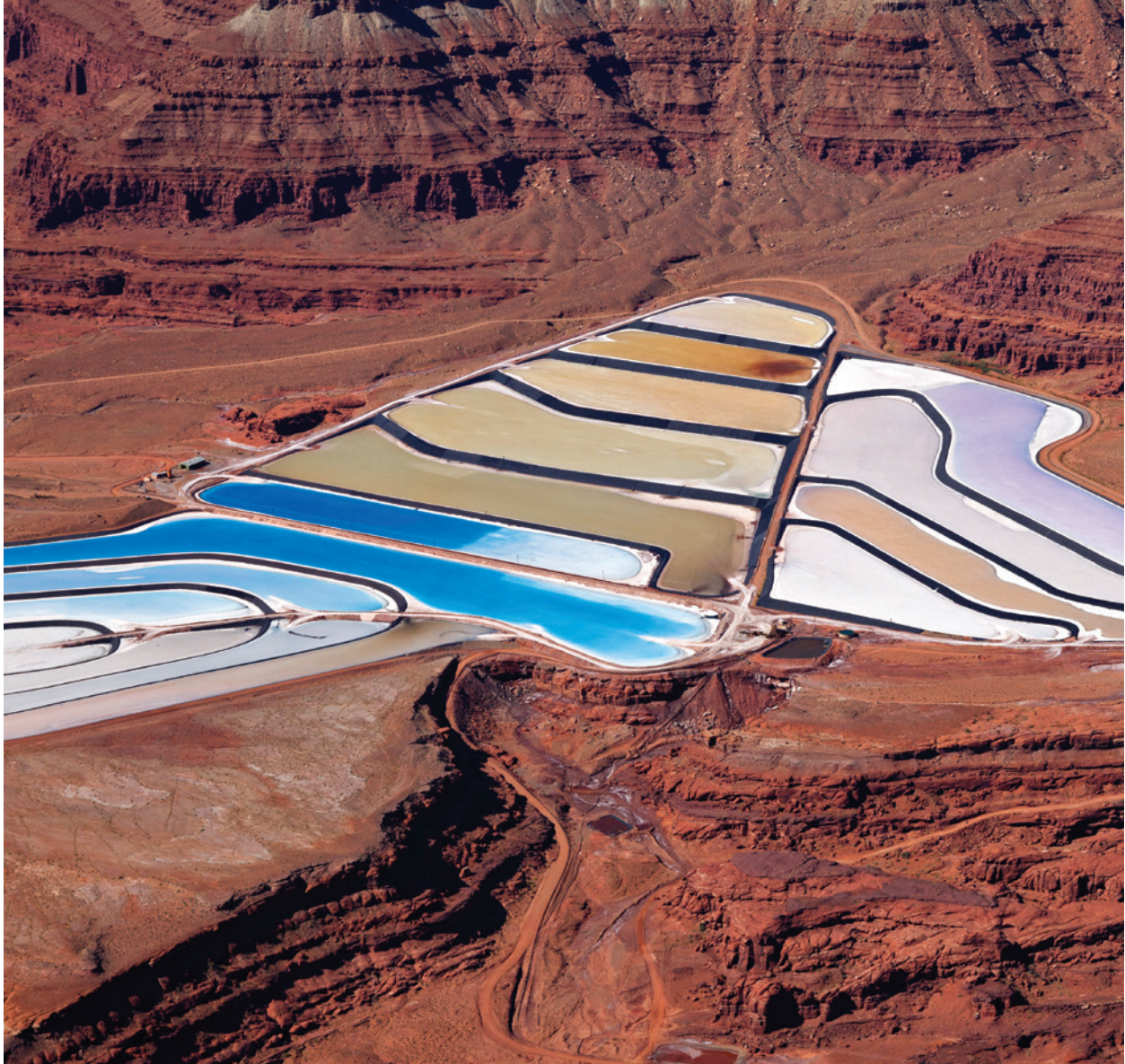
Solar evaporation near Moab, Utah. Solar evaporation involves the use of the sun to evaporate water and precipitate salt in the solution. Photo: Ecoflight
