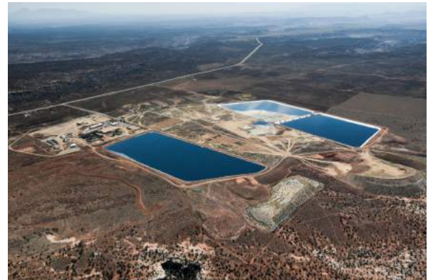
Dom Smith | EcoFlight This aerial photo shot in April shows the White Mesa Uranium Mills evaporation ponds, which environmentalists and Ute Mountain Ute tribal officials fear are emitting radon gas far in excess of federal standards. The 55-acre pond on left is Cell 1, the one with the highest concentrations of radium waste. The mill is six miles south of Blanding on U.S. Highway 191.
