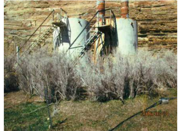
Courtesy | Utah Division of Oil, Gas and Mining Utah state regulators want this long idled well, “operated” by Hot Rod Oil on the East Tavaputs Plateau, plugged and reclaimed. The well has produced no natural gas for the past 13 years and would contaminate nearby water sources if its corroded valves fail, according to the Division of Oil, Gas and Mining. A recent analysis has identified 557 such “orphaned” wells in Utah’s oil fields that have not produced in more than 10 years, yet remain unplugged in defiance of state and federal regulations.
